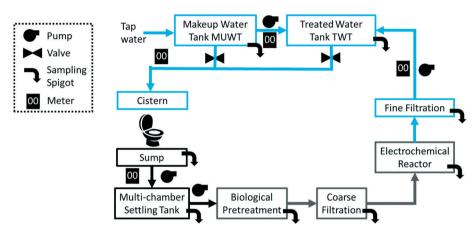
Fig. 1 Flow diagram of the CLASS.
