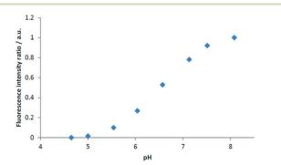
Fig. 4 FITC RB nanosensors calibration in HH Combo medium, normalised fluorescence intensity ratio of IFITC/IRB with varying pH.
