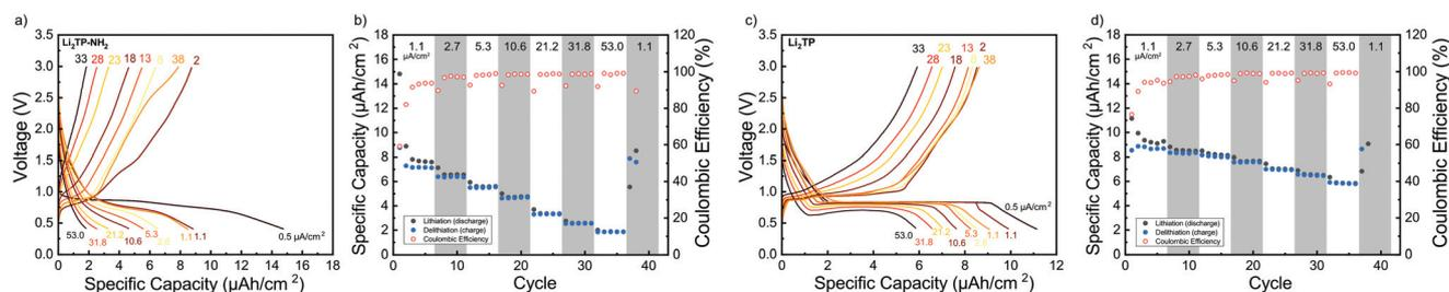
**Fig. 7** Rate capability measurements for Li<sub>2</sub>TP-NH<sub>2</sub> (a and b) and Li<sub>2</sub>TP (c and d): cycling starts with a format cycle with a small current of 0.5 μA cm<sup>-2</sup>, thereafter the current is increased after every 5 cycles before returning to the original value (1.1, 2.7, 5.3, 10.6, 21.2, 31.8, 53.0 μA cm<sup>-2</sup>). In (a) and (c) the shape of the charge–discharge curve at different cycles and in (b) and (d) capacity plotted with coulombic efficiency.
