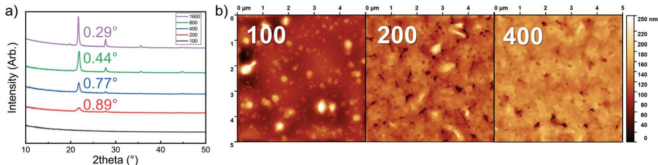
Fig. 3 (a) GIXRD patterns with calculated FWHM values, and (b) AFM images for  $\text{Li}_2\text{TP-NH}_2$  films deposited at 200 °C with increasing number of ALD/MLD cycles. The z-scale in AFM images is 0–50 nm for the sample with 100 cycles and 0–250 nm in samples with 200 and 400 cycles.
