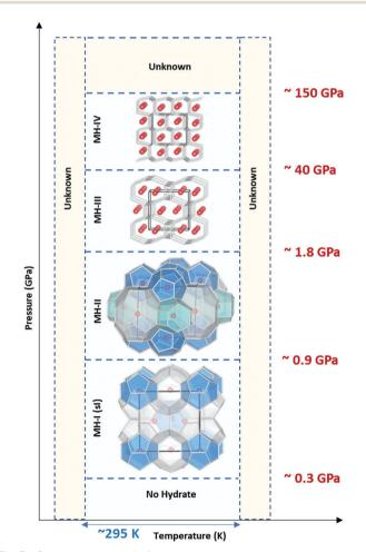
Fig. 3 Structural transition of methane hydrate upon compression up to 150 GPa at room temperature. MH-I is the known sI hydrate. MH-II is similar to sH hydrate and may be closely related to it. However, there are challenging reports about whether MH-II has sH structure or not. 17,32
