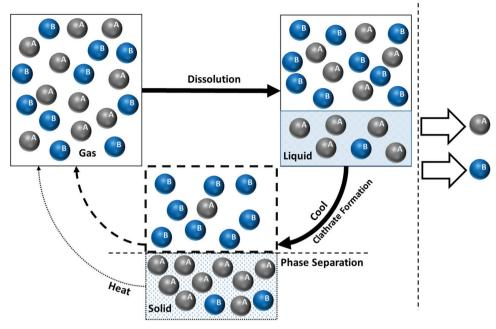
Fig. 29 Schematic diagram of hydrate-based gas separation.
