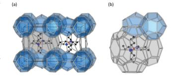
(a) The structure of TBAB hydrate ((C<sub>4</sub>H<sub>9</sub>)4N $^+$ ·Br $^-$ ·38H<sub>2</sub>O). The solid lines represent the unit-cell of each hydrate. (b) Magnification of TBAB hydrate structure near tetra-n-butylammonium cation. The blue shaded dodecahedral cages are empty, and as such are candidates for encaging small molecules.
