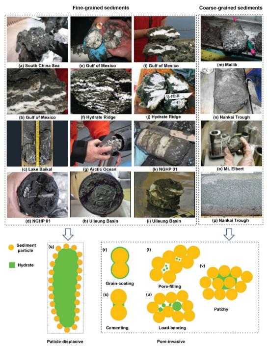
Fig. 8 Core-scale hydrate morphology in HBS samples and conceptual pore-scale habits for fine-grained and coarse-grained sediments (reprinted with permission from Ren et al., 403 Copyright 2020 Elsevier Ltd).
