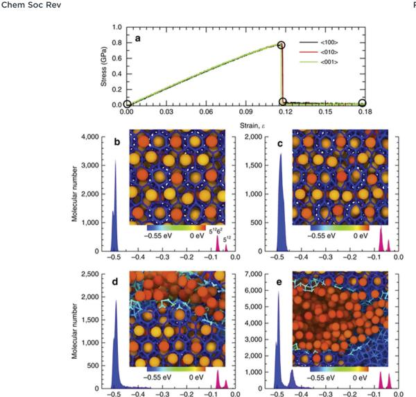
Fig. 7 (a) Stress-strain relationships for single-crystal methane hydrate. The molecular cohesive energy distributions and corresponding localized molecular structures (b) initially, (c) at the onset of fracture, (d) immediately after initial fracture and (e) at a strain of 0.18 (reprinted with permission from Wu et al., 353 Copyright 2015 Springer Nature).
