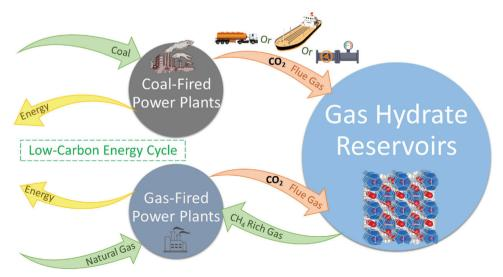
Fig. 24 Illustration of the principal mechanism of the direct injection of flue gas for methane recovery from gas hydrate reservoirs and CO<sub>2</sub> capture and storage simultaneously (adapted with permission from Hassanpouryouzband et al., 81 Copyright 2019 Springer Nature).
