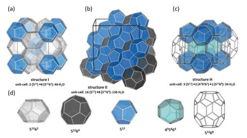
Fig. 2 Three natural gas hydrate structures. (a) Structure I, (b) structure II, and (c) structure H, and (d) five different host water cages. The solid lines represent the unit-cell of each hydrate. All the crystal structures through the review were drawn using a visualization software called "Vesta 3".25
