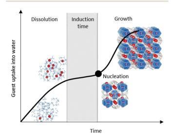
Fig. 10 Typical time dependence of the hydrate crystallization process.
