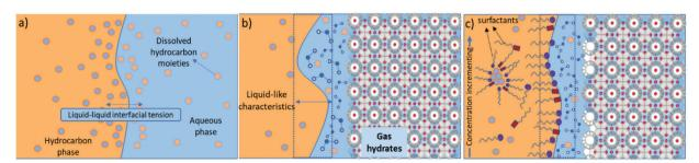
Fig. 9 The various solid hydrate and fluid-fluid interactions which play crucial roles in hydrates crystals formation and inhibitions phenomena; (a) formation of water in oleic phase and hydrocarbon in aqueous phase emulsions; (b) hydrate crystals (solid phase) formation, growth, and their interaction with peripheral water and hydrocarbon molecules at interface; (c) hydrate crystals-water-hydrocarbon molecular interactions in the presence of different surface-active chemical species.
