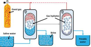
Fig. 28 Schematic diagram of the clathrate hydrate-based desalination process. Seawater is contacted with an appropriate hydrate former such as  $\rm CO_2$  at desired thermodynamic conditions to form clathrate hydrates while excluding salts from the crystalline structure. The hydrate crystal can then be removed from the brine and dissociated to drinking water and hydrate former which could be recycled.
