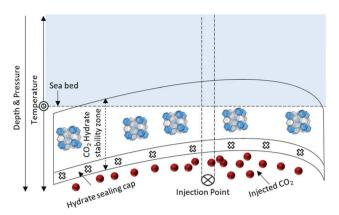
Fig. 25 Schematic diagram of the CO<sub>2</sub> self-sealing mechanism.
