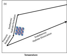
Fig. 27 Two modes of hydrate cold storage technology, namely heating (a) and (b) depressurising for cooling (based on Cheng et al. 920)
