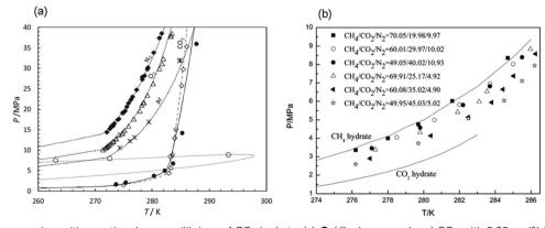
Fig. 23 Effect of common impurities on the phase equilibrium of CO₂ hydrate. (a) ● (○ phase envelope) CO₂ with 5.05 mol% O₂, 2.05 mol% Ar and 3.07 mol% N<sub>2</sub>; ♦ pure CO<sub>2</sub>; ♦ pure N<sub>2</sub>; △ pure O<sub>2</sub>; \* pure Ar; ○ (adapted with permission from Chapoy et al., 1403 Copyright 2013 Elsevier Ltd). (b) CH<sub>4</sub>-CO<sub>2</sub>-N<sub>2</sub> mixtures (adapted with permission from Zang et al., 1404 Copyright 2018 American Chemical Society).
