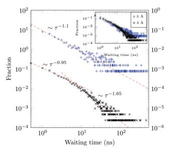
Fig. 13 Normalised frequency of escape events from the circle of radius  $r_{\rm esc}$  in the {x,y}-plane for  $r_{\rm esc}$  = 3 Å (black, left axis) and  $r_{\rm esc}$  = 5 Å (blue, right axis), with  $\tau_{esc}$  = 0.5 ns for both panels. Both distributions are shown together in the inset (sharing the same y-axis).
