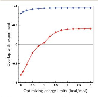
Fig. 6 Fits to the experimental spectra of the two enantiomers of citronellal using the genetic algorithm and the 70 lowest energy conformers of citronellal found within 2 kcal mol<sup>-1</sup> at a BP86/TZP level of theory as a function of the maximum energy modulation  $\Delta \textit{E}^{\text{max}}$ Blue: overlaps from the fit to the correct (S-)enantiomer. Red: overlaps from the fit to the incorrect (R-)enantiomer.
