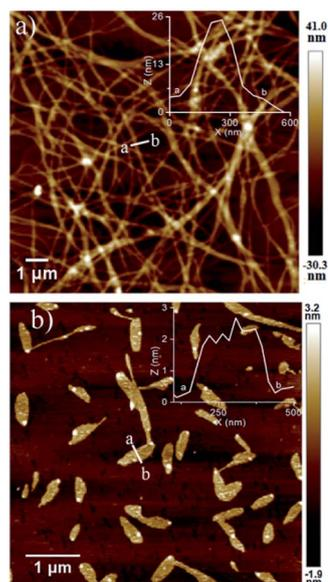
Fig. 4 AFM images of (a) a spontaneous supramolecular polymer produced by NDI-1 in the presence of 10 mol% DMAP and (b) NDI-1<sub>SP</sub> produced by SROP of NDI-1<sub>mono</sub> in the presence of 10 mol% DMAP. In both cases, samples were drop cast on the mica surface at the end of polymerization [ $C = 1 \times 10^{-4}$  M].
