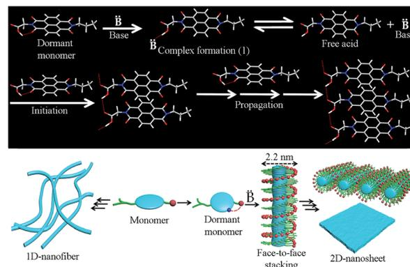
Scheme 1 Top – probable mechanistic pathway for organobase triggered SROP of NDI-1<sub>mono</sub>; bottom – pathway diversity and 2D-assembly of the product produced by SROP.
