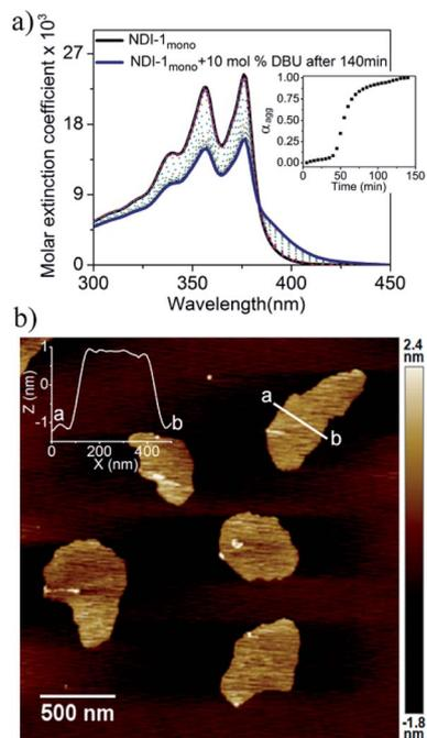
Fig. 2 (a) Time dependent change in the UV/Vis spectra of NDI-1<sub>mono</sub> in the presence of 10 mol% DBU in decane. Inset – variation of  $\alpha_{agg}$  (estimated from the change in  $A_{376\text{ nm}}$ ) as a function of time; (b) AFM image of NDI-1<sub>sp</sub>. Inset: height profile along (a and b).
