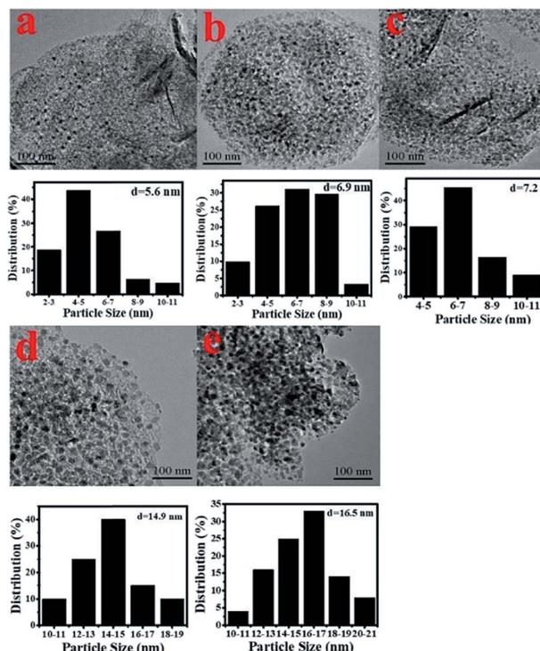
Fig. 3 TEM images of the as-prepared Ni/Al<sub>2</sub>O<sub>3</sub>-*T* catalysts and particle size distribution of the Ni nanoparticles ((a) Ni/Al<sub>2</sub>O<sub>3</sub>-500; (b) Ni/Al<sub>2</sub>O<sub>3</sub>-550; (c) Ni/Al<sub>2</sub>O<sub>3</sub>-600; (d) Ni/Al<sub>2</sub>O<sub>3</sub>-650; (e) Ni/Al<sub>2</sub>O<sub>3</sub>-700).
