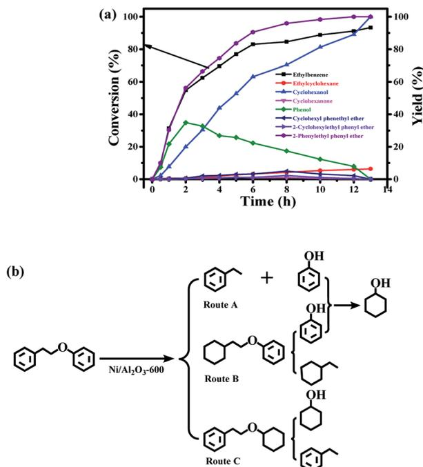
Fig. 7 (a) The time course of the product distributions for the conversion of 2-phenylethyl phenyl ether ( $\beta$ -O-4) over the Ni/Al<sub>2</sub>O<sub>3</sub>-600 catalyst. Reaction conditions: 2-phenylethyl phenyl ether ( $\beta$ -O-4) (198 mg, 1 mmol), Ni/Al<sub>2</sub>O<sub>3</sub>-600 (20 mg), solvent (10 mL), 170 °C, stirring at 1000 rpm, (b) reaction pathway for the cleavage of 2-phenylethyl phenyl ether.
