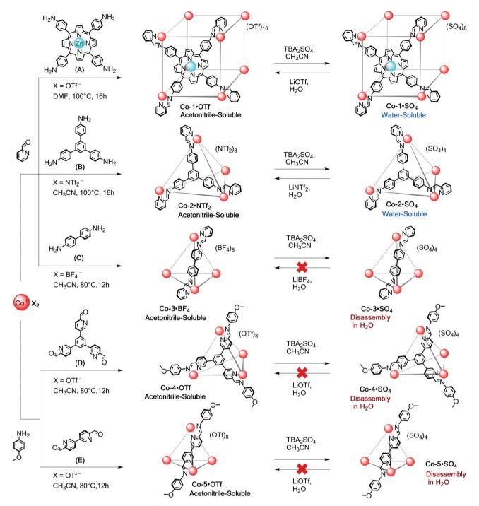
Scheme 1 Subcomponent self-assembly of  $Co^{II}$ -capsules. Preparation of acetonitrile-soluble  $Co-1 \cdot X$  to  $Co-5 \cdot X$  ( $X = OTf^-$ ,  $NTf_2^-$ , or  $BF_4^-$ ) from subcomponents A-E and their anion exchange sequences.
