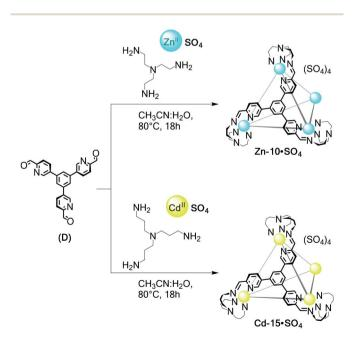
Scheme 5 Self-assembly of water-soluble Zn-10·SO<sub>4</sub> and Cd-15.SO<sub>4</sub> from tritopic subcomponent D.
