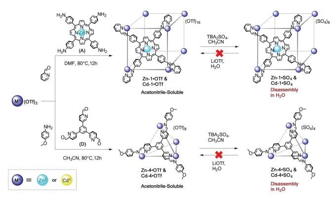
Scheme 4 Self-assembly of face-capped cubic  $\mathbf{1}$  and tetrahedral  $\mathbf{4}$  architectures based on zinc(ii) and cadmium(ii). Sulfate salts of capsules obtained *via* anion exchange from the triflate congeners were observed to disassemble in water. Direct assembly reactions using ZnSO<sub>4</sub> or CdSO<sub>4</sub> did not form the target water-soluble products.
