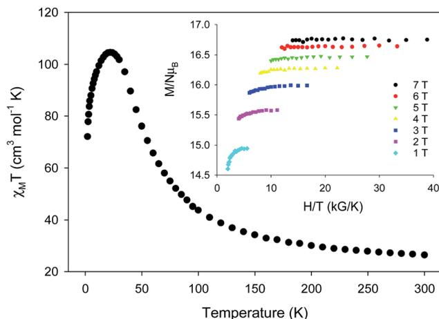
Fig. 2 Temperature dependence of  $\chi_M T$  for **1-d** at 0.1 T. (inset) Magnetization ( $M$ ) versus field ( $H$ ) and temperature ( $T$ ) data, plotted as reduced magnetization ( $M/N\mu_B$ ) versus  $H/T$ , for **1-d** at applied fields of 1–7 T and in the 1.8–5 K temperature range.
