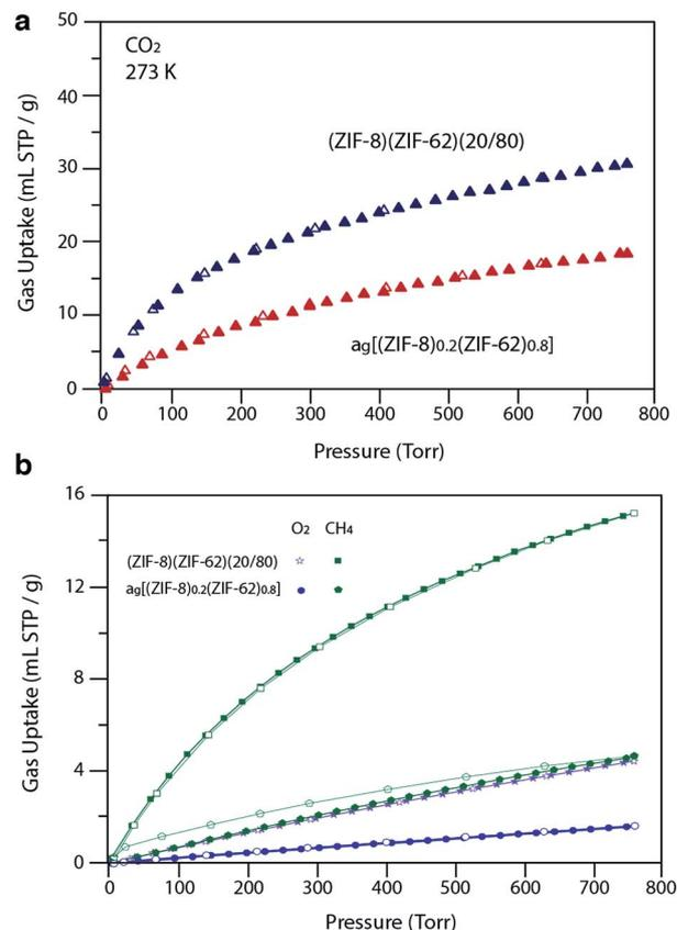
Fig. 7 (a)  $\text{CO}_2$  isotherm at 273 K and (b)  $\text{O}_2$  and  $\text{CH}_4$  at 273 K isotherms for zinc based samples. Closed symbols represent adsorption isotherms and open symbols represent desorption isotherms.
