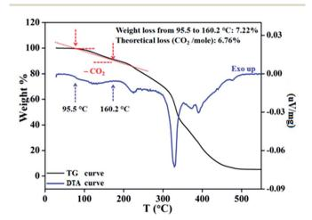
Fig. 3 Removal of captured  $CO_2$  in solid state, as monitored by thermogravimetric-differential thermal analysis of compound 3.
