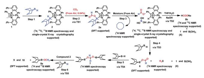
Fig. 6 Mechanistic scheme for the reduction of CO<sub>2</sub> to methoxyborane and sodium formate with 2 in air. For drawings of 9 and 10 see Fig. S3.†
