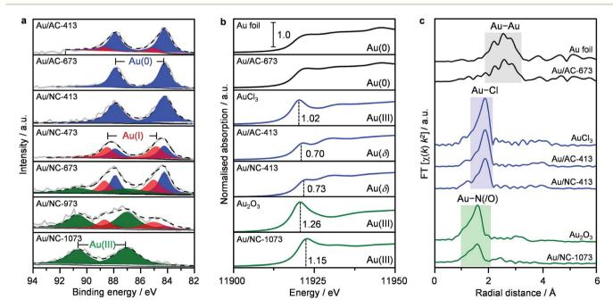
Fig. 2 Analysis of the gold speciation of selected catalysts based on (a) Au 4f XPS, (b) Au  $L_3$  edge XANES, and (c) Fourier transformed EXAFS spectra. Dashed black lines in (a) show the result of fitting the raw data (solid grey lines). Vertical dashed lines in (b) indicate the white line intensity of the distinct cationic gold species. I <  $\delta$  <III.
