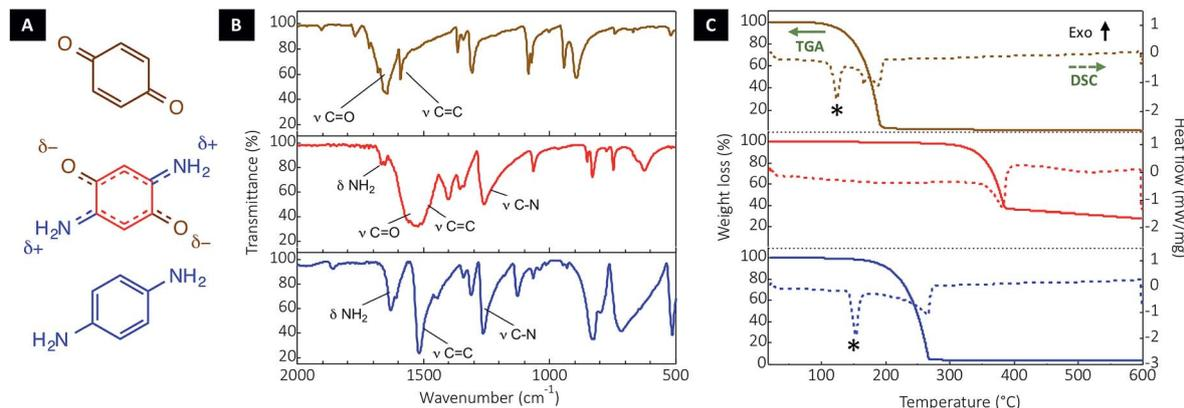
Fig. 2 Stabilization of the DABQ molecular crystal through H-bonding. (A) Molecular structure of DABQ and of the reference compounds (*i.e.*, BQ and *p*-PDA) and their corresponding (B) FTIR spectra as well as (C) thermogravimetry (TG) and differential scanning calorimetry (DSC) plots. The stars mark the melting point in the DSC plots.
