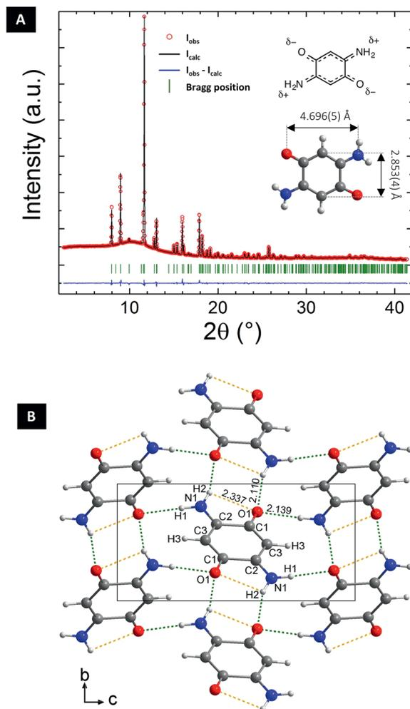
Fig. 1 *Ab initio* structure determination of DABQ. (A) X-ray powder diffraction pattern (final Rietveld refinement) of crystalline DABQ with the molecular structure depicted in the inset. (B) View of the solved DABQ crystal structure (yellow dotted line: intramolecular H-bonds; green dotted line: intermolecular H-bonds).
