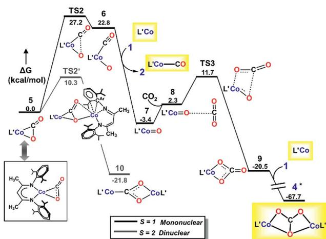
Fig. 6 M06L/def2-TZVPP Gibbs free energy ( $\Delta G$ ) profile for the mononuclear dissociative pathway. Isolated species are shown in yellow boxes, with  $\text{L}'$  depicted instead of  $\text{L}'^{\text{bu}}$ . \*Marked species has lower relative free energy on the  $S = 3$  surface which has been taken to complete the profile.
