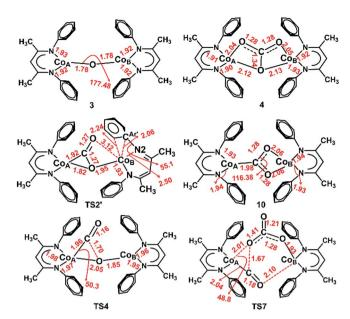
Fig. 8 Optimized structures of 3, 4 and TS2' at the BP86/B1 level of theory and 10, TS4 and TS7 at the B3LYP/B1 level of theory. (See computational details for basis set information and justification of employing the respective methods.) Important interatomic distances (Å) and angles (°) are also shown. Isopropyl groups are omitted for clarity.
