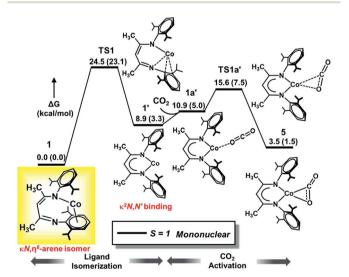
Fig. 4 Computed DLPNO-CCSD(T)/def2-TZVPP Gibbs free energy ( $\Delta G$ ) profile for isomerization of 1 (L'Co) to 1' followed by CO<sub>2</sub> activation. Relative free energy values (in kcal mol<sup>-1</sup>) computed with M06L/def2-TZVPP are given in parentheses. The isolated species is shown in the yellow box, with L' depicted instead of L<sup>fBu</sup>.
