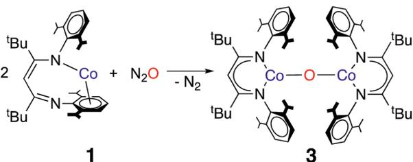
**Scheme 2** Synthesis of **3** from L<sup>tBu</sup>Co and nitrous oxide.
