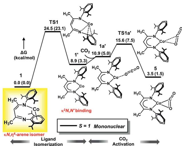
Fig. 4 Computed DLPNO-CCSD(T)/def2-TZVPP Gibbs free energy ( $\Delta G$ ) profile for isomerization of **1** (L'Co) to **1'** followed by CO<sub>2</sub> activation. Relative free energy values (in kcal mol<sup>-1</sup>) computed with M06L/def2-TZVPP are given in parentheses. The isolated species is shown in the yellow box, with L' depicted instead of L<sup>tBu</sup>.
