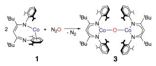
Scheme 2 Synthesis of 3 from L<sup>tBu</sup>Co and nitrous oxide.
