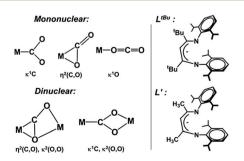
Chart 1 (Left) Different binding modes of CO<sub>2</sub> to mononuclear and dinuclear metal sites. (Right) Actual and truncated ligand frameworks.
