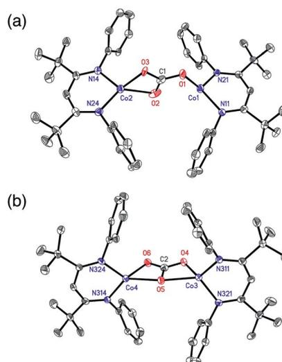
Fig. 1 The two crystallographically independent molecules in the crystal structure of **4**: (a) μ-η<sup>1</sup>:η<sup>2</sup> form, with the major disorder component shown; (b) μ-η<sup>2</sup>:η<sup>2</sup>. H atoms and <sup>i</sup>Pr groups are omitted for clarity. Thermal ellipsoids are shown at 50% probability.
