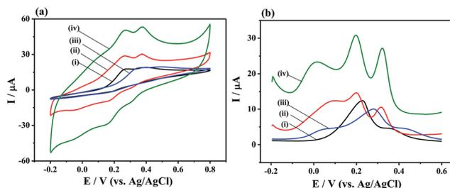
Fig. 3 (a) CV and (b) DPV curves of (i) bare GCE, (ii) MoS<sub>2</sub>/rGO/GCE, (iii) PANI/GCE, and (iv) MoS<sub>2</sub>-PANI/rGO/GCE in 0.1 M PBS (pH 7.0, 0.1 M KCl) containing 2.0 mM AA, 150 μM DA, and 200 μM UA.
