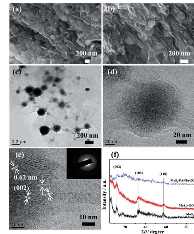
Fig. 2 (a and b) FE-SEM images of  $\text{MoS}_2$ -PANI/rGO nanocomposite; (c) TEM and (d and e) HR-TEM images of 3D  $\text{MoS}_2$ -PANI/rGO nanocomposite (the inset in (e) is the corresponding SAED pattern), and (f) XRD patterns of the  $\text{MoS}_2$ ,  $\text{MoS}_2$ /rGO and  $\text{MoS}_2$ -PANI/rGO samples.
