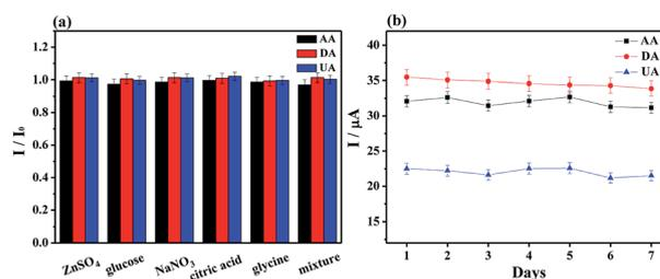
Fig. 7 (a) Peak current ratio of  $\text{MoS}_2\text{-PANI/rGO/GCE}$  to 1.0 mM AA, 75  $\mu\text{M}$  DA, and 75  $\mu\text{M}$  UA in the presence of 1 mM of various interfering substances ( $\text{ZnSO}_4$ , glucose,  $\text{NaNO}_3$ , citric acid, glycine, and the mixture, respectively). (b) The stability of  $\text{MoS}_2\text{-PANI/rGO/GCE}$  in 0.1 M PBS (pH 7.0, 0.1 M KCl) containing 1.0 mM AA, 75  $\mu\text{M}$  DA, and 75  $\mu\text{M}$  UA.
