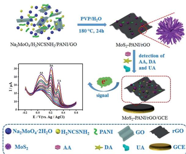
Scheme 1 Schematic diagram of MoS<sub>2</sub>-PANI/rGO-based electrochemical biosensor for simultaneous detection of AA, DA, and UA.
