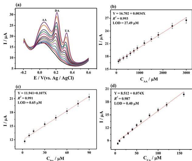
Fig. 6 (a) DPV curves of  $\text{MoS}_2\text{-PANI/rGO/GCE}$  in 0.1 M PBS (pH 7.0, 0.1 M KCl) containing AA, DA, and UA with different concentrations. The concentration from bottom to top: 30  $\mu\text{M}$  to 3.0 mM for AA, 3.0 to 300  $\mu\text{M}$  for DA, and 2.0 to 200  $\mu\text{M}$  for UA, respectively. The plots of the oxidative peak currents versus the concentrations of (b) AA, (c) DA, and (d) UA.
