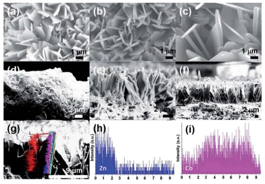
Fig. 2 Microstructure and elemental distribution of ZIF-L membranes: (a and d) Co-ZIF-L, (b and e) Zn-ZIF-L, (c and f) Zn/Co-ZIF-L, (q-i) element distributions of Zn and Co.
