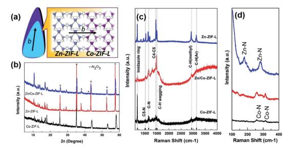
Fig. 3 Structural characterization of ZIF-L membranes. (a) Schematic illustration of the crystal structure for the heterogeneous growth of Co-ZIF-L on Zn-ZIF-L along b-axis. (b) XRD patterns of homogeneous membranes (Zn-ZIF-L and Co-ZIF-L) and heterogeneous membranes (Zn/ Co-ZIF-L) grown on porous ceramic supports. (c and d) Raman spectra of Zn-ZIF-L, Co-ZIF-L and Zn/Co-ZIF-L samples collected from the corresponding membranes.
