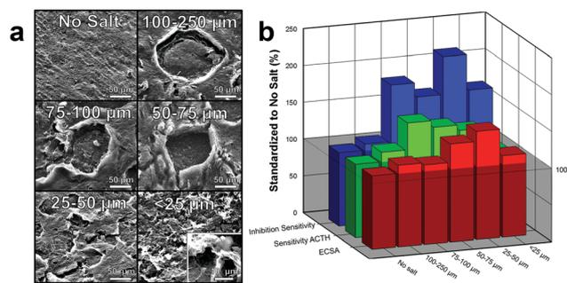
Fig. 4 Effects of various size salt crystals for macroscale pore formation. (a) SEM depicting various size salt pores made with decreasing size salt crystals. Bottom right: Magnification of <25  $\mu\text{m}$  pore. (b) Graph demonstrated the effects of different size salt crystals to ECSA (red), sensitivity to 5 mM ACTH (green), and inhibition sensitivity due to 1  $\mu\text{M}$  paraoxon (blue). Note: graph has been standardized to no salt pores for comparison.
