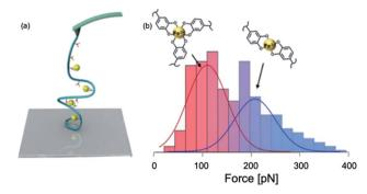
Schematics of SMFS study on catechol-Fe<sup>3+</sup> complex (a) and force spectroscopy (b). Reprinted with permission from ref. 100. Copyright (2017) American Chemical Society.
