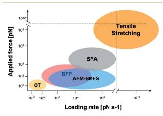
Fig. 2 Force and loading rate ranges of different force measurement approaches. OT represents optical tweezers and its range is estimated from ref. 42–44. Bio-membrane force probe (BFP) is estimated from ref. 45. AFM-based SMFS data are from ref. 46–48 and are estimated by general AFM technical details and typical cantilever mechanical properties. SFA data are from ref. 33, 49 and 50. Tensile stretching data are estimated from ref. 47 and 51–54.
