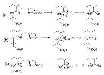
Fig. 22 Possible interaction mechanisms between the acrylate components and solvent molecules in the acrylic gel polymer electrolytes for the  $\rm H_2SO_4/PAMPS$  electrolyte. This figure has been adapted from ref. 206 with permission from Elsevier.
