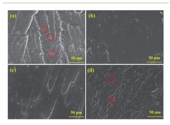
Fig. 5 Cross-sectional morphology of coatings: (a) pure EP; (b) 0.5% N-CDs-EP; (c) 1.0% N-CDs-EP; (d) 2.0% N-CDs-EP.
