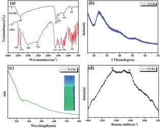
Fig. 3 (a) Fourier transform infrared (FTIR) spectra, (b) XRD pattern of N-CDs, (c) UV-vis absorption spectra of N-CDs and (d) Raman spectrum.
