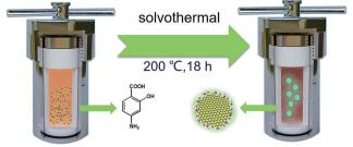
Fig. 1 Schematic illustration of the preparation of N-CD nanomaterials.
