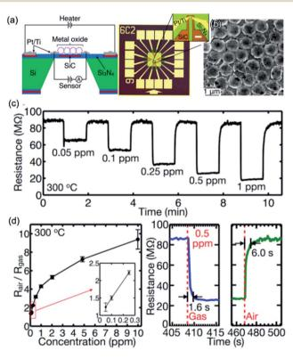
Fig. 7 (a) Schematic diagram and (b) morphology of the as-fabricated sensor with the integration of microheater platform and macroporous  $\rm SnO_2$  hollow spherical array. (c) Real-time sensor resistance transient to HCHO at 300 °C. (d) Sensor response  $\it versus$  HCHO concentration, and real-time sensor response and recovery behaviors to 0.5 ppm HCHO. Reproduced with permission.  $^{84}$  Copyright 2017, American Chemical Society.
