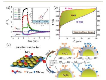
Fig. 8 (a)  $NO_2$  response of 2DOM  $Fe_2O_3$  at different temperatures (T) and concentrations (C). (b) T-C transition phase diagram. (c) Schematic illustration of different  $NO_2$  sensing types at high and low C values, respectively. Reproduced with permission. P8 Copyright 2015, Royal Society of Chemistry.
