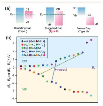
Fig. 9 (a) Three types of semiconductor heterojunctions organized by band alignment. (b) CB and VB band positions referred to the Fermi level  $(E_C - E_F)$  or  $E_V - E_F$ ). In the upper portion, the CB position is arranged according to the distance to  $E_{\rm F}$  for these oxides; in the bottom part, the VB position is also arranged according to the distance to  $E_{\rm F}$ .
