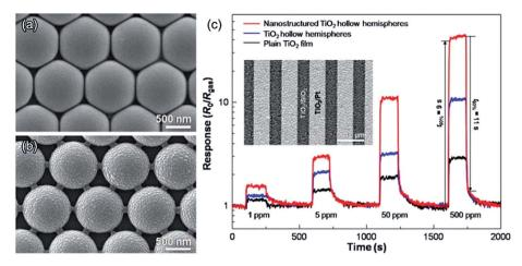
Fig. 6 Top-view SEM images of (a)  $TiO_2$  hollow hemispheres and (b) nanostructured  $TiO_2$  hollow hemispheres (pointy contact between hemispheres); (c) sensing transients of plain  $TiO_2$  film, hollow hemispheres, and nanostructured hollow hemispheres to 1–500 ppm CO at 250 °C. Reprinted with permission.<sup>82</sup> Copyright 2010, Elsevier Ltd.
