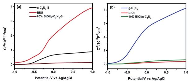
Fig. 6 Mott–Schottky plots for (a) pristine  $g-C_3N_4-S$ , pristine BiOl and  $g-C_3N_4-S$ /BiOl and (b) pristine  $g-C_3N_4$ , pristine BiOl and  $g-C_3N_4$ /BiOl. The plots are shown in two different figures with two different scales (vertical axis) for improved visibility.
