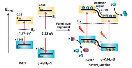
Fig. 8 Proposed mechanism of charge separation in g-C<sub>3</sub>N<sub>4</sub>-S/BiOI heterostructured photoanodes
