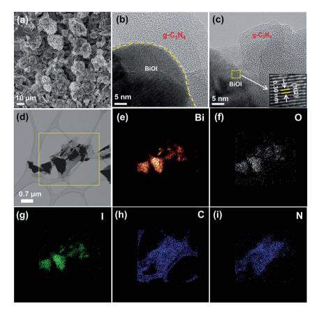
Fig. 3 (a) FESEM image of  $q-C_3N_4-S/BiOI$  thin film and HR-TEM of  $q-C_3N_4-S/BiOI$  images at (b) 5 nm scale bar showing heterojunction of BiOI and  $g-C_3N_4-S$ , (c) at 5 nm scale bar showing lattice fringes and insets shows d-spacing corresponding to  $g-C_3N_4-S$  and BiOI, (d) bright field STEM image of g-C<sub>3</sub>N<sub>4</sub>-S/BiOI, and STEM elemental mapping for (e) Bi, (f) O, (g) I, (h) C, (i) N.
