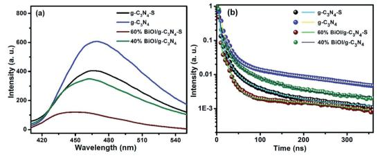
Fig. 7 (a) Steady state PL spectra ( $\lambda_{exc} = 330$  nm) for pristine  $g-C_3N_4-S$ , pristine  $g-C_3N_4$ , pristine BiOI,  $g-C_3N_4-S/B$ iOI and  $g-C_3N_4/B$ iOI. The PL spectrum of BiOI was very weak and is not shown. (b) Time resolved photoluminescence spectra ( $\lambda_{exc} = 405$  nm) and (b) Raman spectra ( $\lambda_{exc} = 780$  nm) of pristine  $g-C_3N_4-S$ , pristine  $g-C_3N_4-S/B$ iOI and  $g-C_3N_4/B$ iOI heterostructures.
