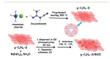
Fig. 1 Synthetic strategy of q-C<sub>3</sub>N<sub>4</sub>-S/BiOI heterojunction composite.
