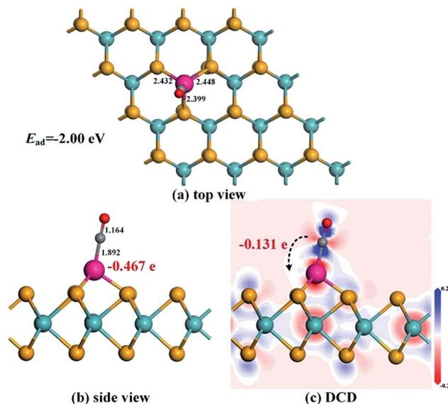
Fig. 3 Adsorption configuration (a) and (b) and DCD (c) of the Rh-MoSe<sub>2</sub>/CO system.
