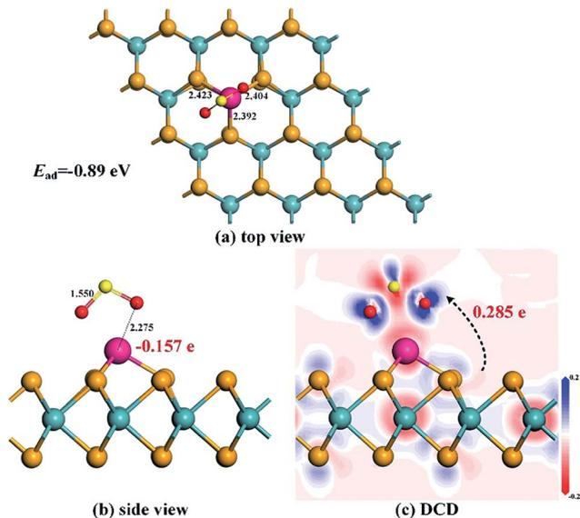
Fig. 9 Adsorption configuration (a) and (b) and DCD (c) of the Rh-MoSe<sub>2</sub>/SO<sub>2</sub> system.
