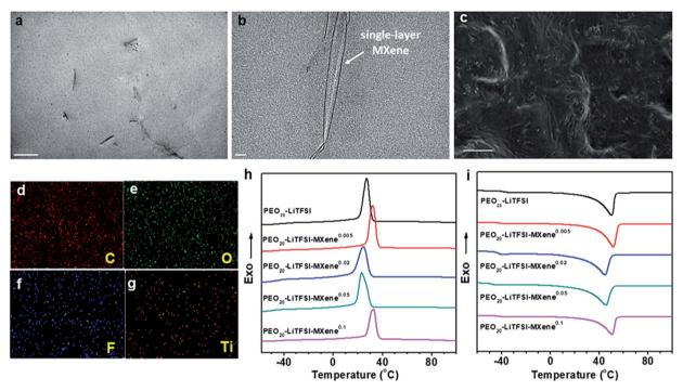
Fig. 2 TEM micrographs of the cross-section of PEO<sub>20</sub>-LiTFSI-MXene<sup>0.02</sup> ((a), scale bar is 500 nm; (b), scale bar is 20 nm). SEM image ((c), scale bar is 3 µm) and SEM-EDS surface scan of C (d), O (e), F (f) and Ti elements (g) in the cross-section of PEO<sub>20</sub>-LiTFSI-MXene<sup>0.05</sup>. DSC thermograms obtained at a rate of 10 °C min<sup>-1</sup> during first cooling (h) and second heating (i).
