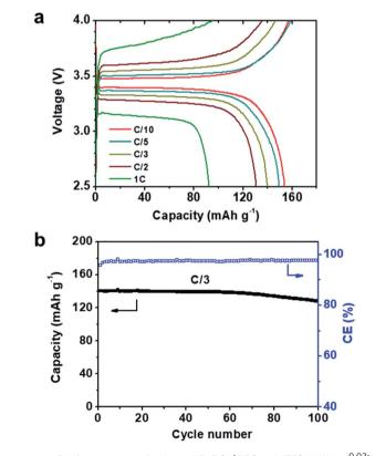
Fig. 4 Performance of the LiFePO<sub>4</sub>|PEO<sub>20</sub>-LiTFSI-MXene<sup>0.02</sup>|Li battery at 60 °C. (a) Voltage profile at different C rates. (b) Capacity and coulombic efficiency vs. cycle number at C/3. The LiFePO<sub>4</sub> loading is  $\approx 2.88$  mg cm<sup>-2</sup>.
