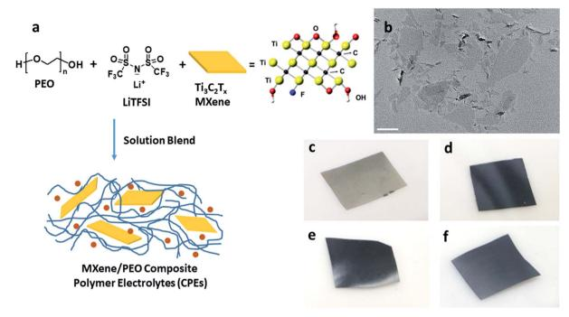
Fig. 1 Fabrication of MCPEs. (a) Preparation procedure of MCPEs. (b) TEM micrograph of the as-prepared few-layer MXene, scale bar is 100 nm. (c-f) Photographs of the MCPE membranes, (c)  $PEO_{20}$ -LiTFSI-MXene<sup>0.005</sup>, (d)  $PEO_{20}$ -LiTFSI-MXene<sup>0.02</sup>, (e)  $PEO_{20}$ -LiTFSI-MXene<sup>0.05</sup> and (f)  $PEO_{20}$ -LiTFSI-MXene<sup>0.1</sup>.
