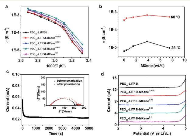
Fig. 3 (a) Temperature scan of the ionic conductivities of the MCPEs. (b) Ionic conductivities vs. MXene content at 28 °C and 60 °C. (c) Lithium transference number measurement of the PEO<sub>20</sub>-LiTFSI-MXene<sup>0.02</sup>. (d) Linear sweep voltammetry of the MCPEs (scan rate  $0.1 \text{ mV s}^{-1}$ ). Curves are shifted along the current axis for clarity.
