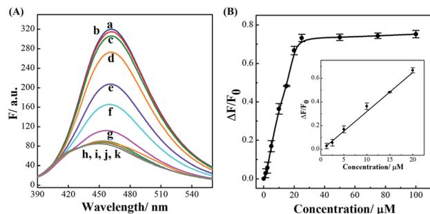
Fig. 6 (A) Fluorescence spectra of the CDs in the presence of BDBA and various concentration of glucose: (a) 0, (b) 1.25, (c) 2.5, (d) 5, (e) 10, (f) 15, (g) 20, (h) 25, (i) 50, (j) 75, and (k) 100  $\mu\text{M}$ . (B) Calibration curve corresponding to the fluorescence response of various concentrations of glucose by BDBA-mediated CDs.  $F_0$  and  $F$  represent the fluorescence intensity in the absence and presence of glucose, respectively. Error bars were derived from  $n = 3$  experiments.
