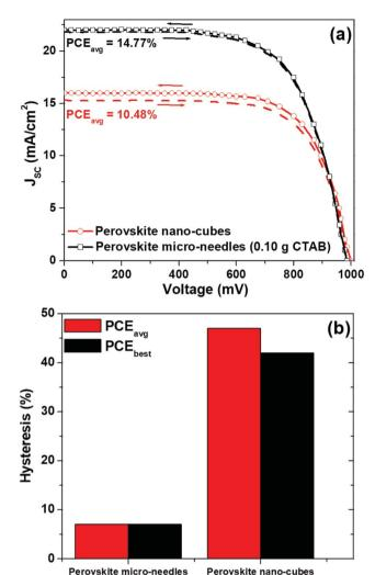
Fig. 4 (a) Comparison of J-V plots of perovskite devices based on MAPbl<sub>3</sub> micro-needles and nano-cubes, and (b) hysteresis for devices with MAPbI<sub>3</sub> micro-needles and nano-cubes, respectively
