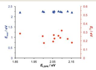
Fig. 4 Variation in the exciton energy (triangles) and scaled coupling energy (circles) as a function of the LSPR energy for a monolayer of LHCII attached to gold nanostructures.
