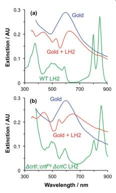
Fig. 7 Extinction spectra for arrays of gold nanostructures before (blue) and after (red) attachment of (a) WT LH2 and (b) the \( \Delta crtl::crtl^{Pa} \) \( \Delta crtC \) mutant of LH2 from \( R. \) sphaeroides. Absorption spectra of the proteins in solution are shown in green.
