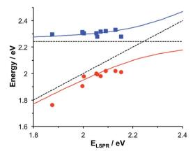
Fig. 3 Dispersion curves for the plexcitonic states determined from experimental data (circles and squares) together with curves fitted using eqn (1). The dotted lines represent the energies of the uncoupled exciton and LSPR states.
