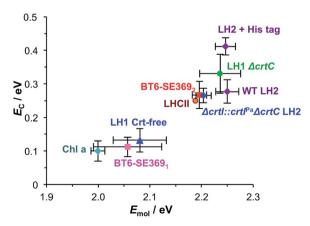
Fig. 6 Mean coupling energy  $E_{\rm C}$  as a function of the exciton energy  $E_{\rm mol}$  for a variety of light-harvesting complexes and for self-assembled monolayers derivatised by attachment of chlorophyll a. For LHCII, the error bars are similar in size to the symbol used.
