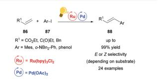
Scheme 33 Ligand-free, visible-light promoted palladium-catalysed Heck cross-coupling. Reagents and conditions: olefin 86 (2.00 equiv.), aryl iodide 87 (1.00 equiv.), Ru-photocat. (1.0 mol%), Pd-cat. (1.0 mol%), Et<sub>3</sub>N (2.00 equiv.), DMF, rt, blue LED. 116
