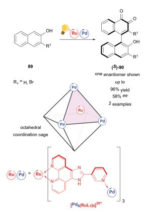
Scheme 34 Coordination cage-catalyzed naphthol photo-hydrogen-evolving unit shown as a catalyst. Reagents and conditions: naphthol 89 (1.00 equiv.), Ru/Pd-photocat. (10.0 mol%), D2O, rt, air, blue LED (8 W), 24 h. 117
