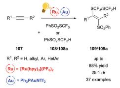
Scheme 41 Atom transfer radical addition for a stereoselective thiosulfonylation. Reagents and conditions: alkyne 107 (1.00 equiv.), PhSO<sub>2</sub>SCF<sub>3</sub> 108 or 108a (1.10 equiv.), Ru-photocat. (2.5 mol%), Au-cat. (0.5 mol%), MeOH/DMF (1/9), rt, white LED (13 W), 2 h. 134
