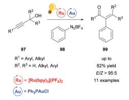
Scheme 37 Tandem arvlative Meyer-Schuster rearrangement. Reagents and conditions: propargyl alcohol (1.00 equiv.), PhN<sub>2</sub>BF<sub>4</sub> 98 (4.00 equiv.), KH<sub>2</sub>PO<sub>4</sub> (4.00 equiv.), Ru-photocat. (2.5 mol%), Au-cat. (10.0 mol%), MeOH, rt, Ar, 5 W green LED, 16 h.<sup>123,126</sup>
