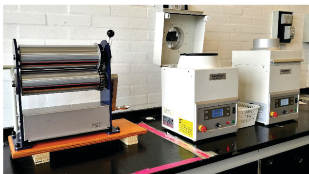
Fig. 9 Laboratory-scale mixers. From the left: roll mill with two rolls and two speed mixers. Optimised mixing is required for reliable elastomers, and for most silicone elastomer formulations high shear mixing is strictly required.
