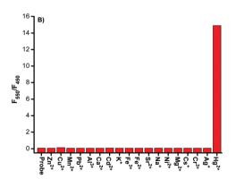
Fig. 2 (A) Fluorescence spectra of probe NAP-PS (10  $\mu\text{M})$  before and after the addition of 200  $\mu$ M different metal ions in HEPES buffer (1.0 mM, pH = 7.4),  $\lambda_{\rm ex}$  = 380 nm, slits: 3/5 nm; (B) fluorescence intensity ratios ( $F_{550}/F_{450}$ ) of probe NAP-PS (10  $\mu$ M) before and after the addition of 200  $\mu$ M different metal ions in HEPES buffer (1.0 mM, pH = 7.4).
