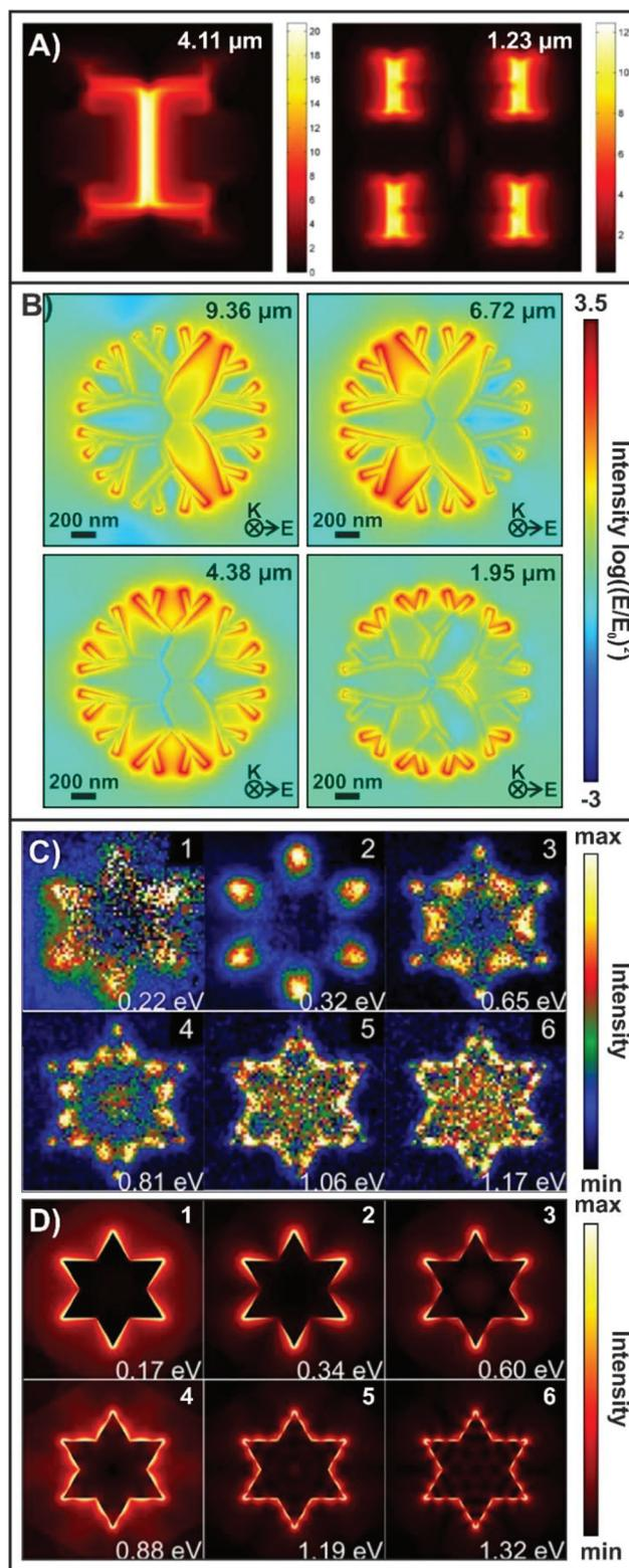
**Fig. 5** EM field distributions for (A) an H-tree fractal,<sup>87</sup> and (B) a three-branched fourth-order generation dendritic fractals.<sup>59</sup> (C) Experimental EELS maps and (D) corresponding calculated EM field maps for a first-order generation Koch fractal.<sup>86</sup> Reproduced and adapted with permission from ref. 87, 59, and 86. Copyrights 2013 IOP Publishing and 2017 American Chemical Society respectively.
