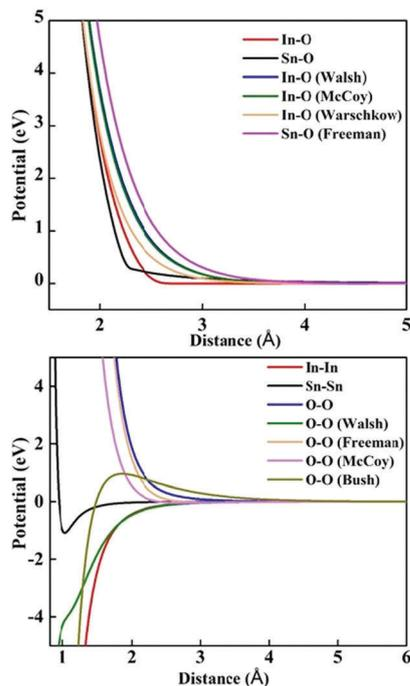
Fig. 2 Interatomic potential model for  $\text{In}_2\text{O}_3$  and  $\text{SnO}_2$ . Metal–oxygen interactions are shown in the top panel, while metal–metal and oxygen–oxygen interactions are shown in the bottom panel. Our model is compared with other previously published ones (see the text for details).
