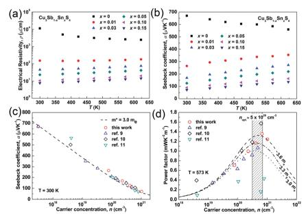
Fig. 5 (a) Electrical resistivity and (b) Seebeck coefficient as functions of temperature; (c) Seebeck coefficient and (d) power factor as functions of carrier concentration in Cu<sub>3</sub>Sb<sub>1-x</sub>Sn<sub>x</sub>S<sub>4</sub> system
