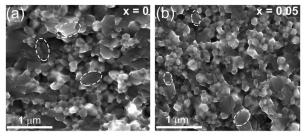
**Fig. 3** Representative SEM images of fractured surface for  $Cu_3Sb_{1-x}Sn_xS_4$ , (a) x=0, (b) x=0.05. Striation-like defects were observed on the transgranular fracture of the grains.
