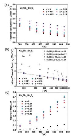
Fig. 8 (a) Thermal conductivity, (b) lattice thermal conductivity and (c) zT values of as functions of temperature in  $Cu_3Sb_{1-x}Sn_xS_4$  system.
