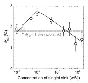
Fig. 5 UC quantum yield of DPA/PtOEP/PE singlet sink/PMMA films ( $c_{\text{DPA}}=25$  wt%,  $c_{\text{PtOEP}}=0.01$  wt%) as a function of singlet sink concentration. The solid line is a guide to the eye. The dashed line indicates the maximum  $\Phi_{\text{UC}}$  of the corresponding material without the singlet sink. The error bars were derived by averaging data of three samples.
