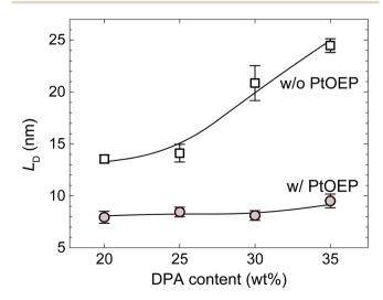
Fig. 3 Singlet exciton diffusion length as a function of DPA concentration in DPA/PMMA films with (circles,  $c_{\text{PtOEP}} = 0.05$  wt%) and without (squares) PtOEP sensitizer. Lines are guides to the eye.
