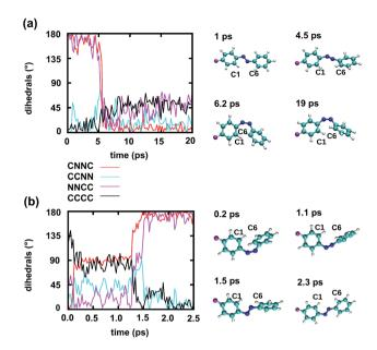
Fig. 6 Time dependence of different dihedrals for a reactive trajectory of the Azo-RNA1 complex, starting from (a) *trans* azobenzene and (b) *cis* azobenzene, along with snapshots of the relevant azobenzene structures. Note that the CNNC and NNCC dihedrals are strongly correlated during the isomerisation event.
