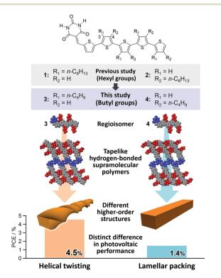
Fig. 1 Molecular structures of barbiturated oligothiophenes 1, 2, 3, and 4, and their hydrogen-bonded motifs and self-assembled nanostructures of 3 and 4 with the best PCEs of the optimized BHJ solar cells.
