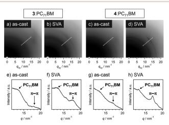
Fig. 6 (a-d) GI-XRD images of (a and b) 3:PC71BM and (c and d) 4:PC<sub>71</sub>BM films. Images (a and c) were taken in the as-prepared state, and images (b and d) were taken after SVA using CS2 for 80 s. (e-h) Radial profiles along the direction shown by white dashed lines in images (a-d), respectively, to pick up diffractions associated with  $PC_{71}BM$  and  $\pi-\pi$  stacked oligothiophene moieties.
