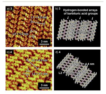
Fig. 2 (a and c) STM images of (a) 3 and (c) 4 at the 1-phenyloctane–HOPG interface. Tunneling current ( $l_t$ ) = 9 pA, bias voltage ( $V_s$ ) = +0.65 V. The concentration of the solution is 5  $\times$  10<sup>-6</sup> M. (b and d) Molecular models of two-dimensionally arranged tapelike supramolecular polymers of (b) 3 and (d) 4 based on the STM images.
