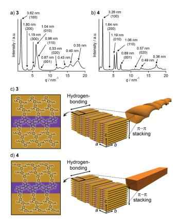
Fig. 4 (a and b) PXRD patterns of precipitates formed from the toluene solution of (a) 3 and (b) 4 in a glass capillary (diameter: 1.0 mm). Values in parenthesis denote Miller indices. (c and d) Schematic representation of the proposed packing structures of (c) 3 in helical nanofibers and (d) 4 in lamella.
