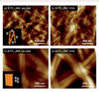
Fig. 5 (a–d) AFM images of (a and b)  $3:PC_{71}BM$  and (c and d)  $4:PC_{71}BM$  films (a and c) before and (b and d) after SVA using CS<sub>2</sub> for 80 s. Inset of (a) and (c): schematic illustration of the morphologies of  $3:PC_{71}BM$  and  $4:PC_{71}BM$ .
