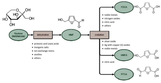
Fig. 7 Catalytic oxidation of HMF into acids.
