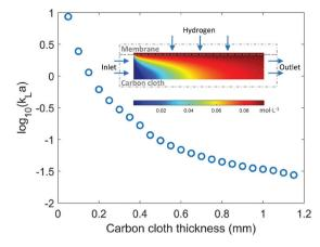
Fig. 3 The mass transfer coefficient  $k_L a$  values under various carbon cloth thicknesses. Insert figure: the hydrogen concentration profile in the membrane and carbon cloth (membrane thickness is 40  $\mu$ m, and carbon cloth thickness is 0.6 mm).
