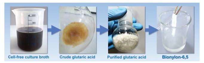
Fig. 6 Downstream purification of bio-based glutaric acid and polymerization into nylon-6,5. Crude glutaric acid was recovered from the broth by a two-step acidification and vacuum concentration procedure. Purified glutaric acid was obtained by crystallization. The bio-based glutaric acid was activated with oxalyl chloride and was then used to perform interfacial polycondensation with 1,6-hexamethylene diamine into nylon-6,5.
