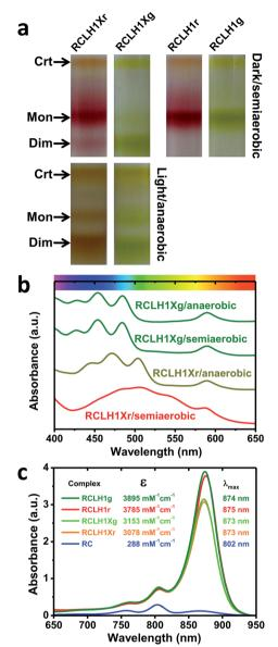
Fig. 2 A variety of RCLH1 complexes from *Rba. sphaeroides*. (a) Bands formed by pigment-proteins separated on sucrose density gradients, (b) visible region absorbance spectra for the RCLH1Xr and RCLH1Xg complexes, (c) molar absorption coefficients for the purified RCLH1(X) or RC complexes and near-IR absorbance spectra for 1  $\mu$ M solutions.
