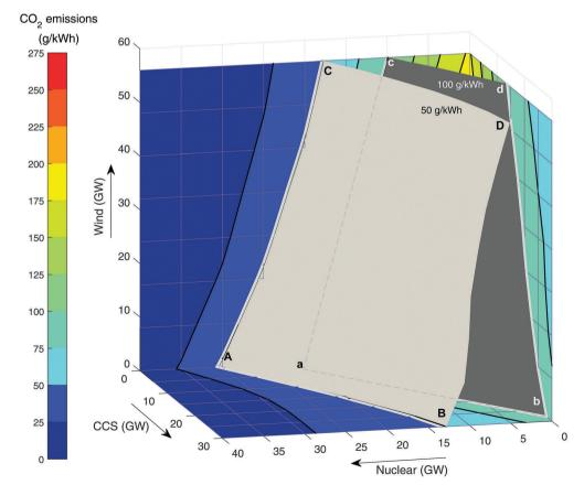
Fig. 5 The CO<sub>2</sub> emissions as a function of nuclear, CCS and wind build. The surfaces show the technology deployment requirements in order to meet the CCC targets for CO<sub>2</sub> emissions of 100 g kWh<sup>-1</sup> and 50 g kWh<sup>-1</sup>.
