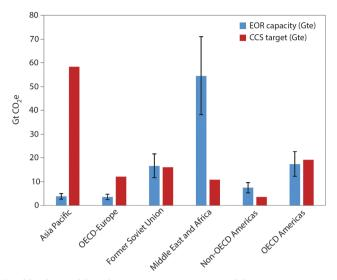
Fig. 20 Global  $\rm CO_2$ -EOR capacity compared with  $\rm CO_2$  mitigation targets. Figure reproduced from Mac Dowell *et al.*  $^{967}$  Data from Dooley *et al.*  $^{974}$  IEA,  $^{975}$  and CIA.  $^{976}$  The error bars indicate an average calculated variance of 30%. The actual reported variance is in the range of 25–35%.
