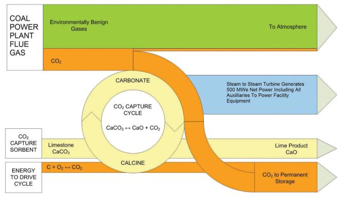
Fig. 10 Schematic of the calcium looping (CaL) cycle.
