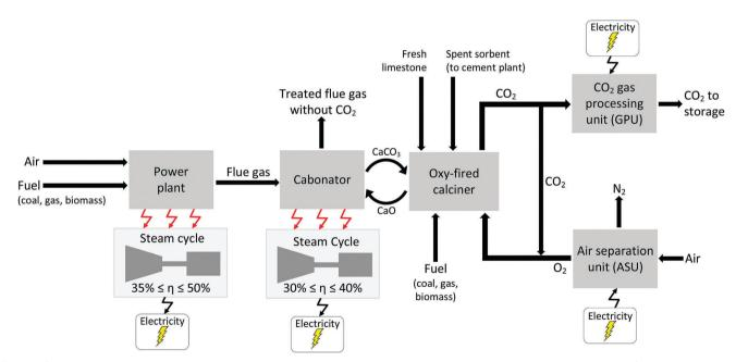
Fig. 11 Calcium looping within a post-combustion capture process. Note that some units of operation may generate power (e.g., the carbonator), whereas the GPU and ASU requires a power supply.
