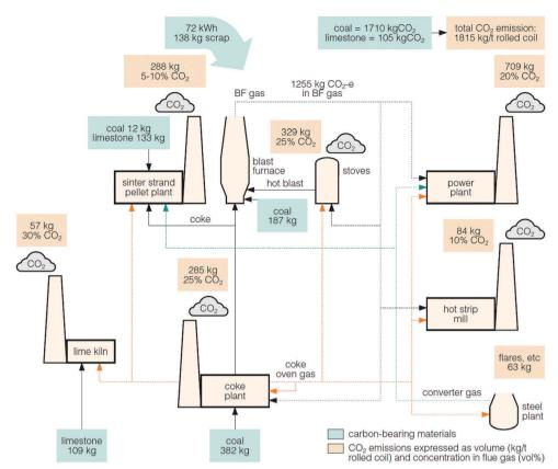
Fig. 8 A typical steel mill and the  $CO_2$  emissions, which vary in concentration. <sup>117,118</sup>
