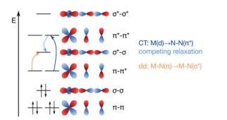
Fig. 3 Two theoretical pathways relevant to dinitrogen photocleavage according to Fischler and von Gustorf for an Fe- $\eta^1$ -N $_2$  complex (metal d-electrons not specified). Orange:  $M-N(\pi)$  to  $M-N(\sigma^*)$  excitation; dark blue: M(d) to N-N( $\pi^*$ ) excitation, shown here as M(d) is the M-N( $\pi^*$ ) orbital; light blue: competing relaxation into  $M-N(\sigma^*)$ . 55
