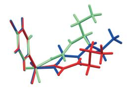
Fig. 2 Overlay of the asymmetric CPA molecule in the  $\alpha$ -CPA (blue), β-CPA (red), and ε-CPA (green).
