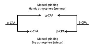
Fig. 4 Schematic influence of humidity on CPA phase conversion. Both forms convert to  $\alpha\text{-CPA}$  when manually ground under a humid atmosphere. No conversion is found under dry atmosphere.
