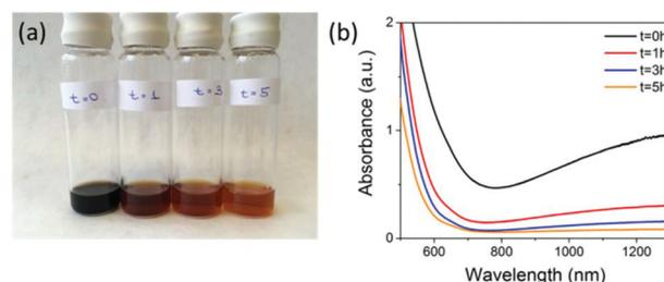
Fig. 1 (a) Picture showing 5 mL aliquots taken from the reaction mixture at (from left to right)  $t = 0, 1, 3$  and 5 hours post-exposure to air. (b) The corresponding loss of absorbance above ~650 nm for the aliquots removed from the reaction mixture.
