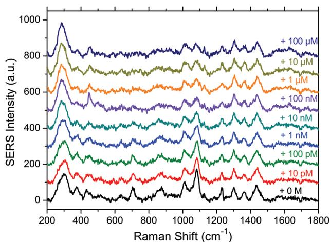
Fig. 3 Average SERS spectra for each OTA concentration. Bottom black curve is the null concentration, and then the concentration increases for stacked spectra up to  $100\text{ }\mu\text{M}$  for the top dark blue spectrum.
