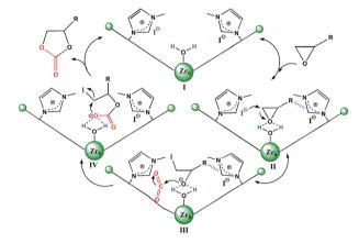
Scheme 2 Plausible mechanism of 2 catalyzed cycloaddition reaction of  $CO_2$  with epoxides. The hashed bonds represent  $\pi \cdots \pi$ , cationic $\cdots \pi$  or hydrogen bonding interactions.
