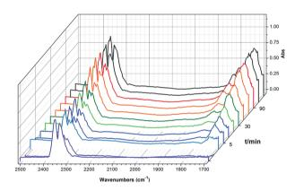
Fig. 3 In situ FT-IR spectra of the synthesis of chloropropene carbonate catalyzed by 2 at  $100\,^{\circ}$ C under an atmospheric dilute  $CO_2/N_2$  gas mixture. IR absorption of 2 is subtracted for clarity.
