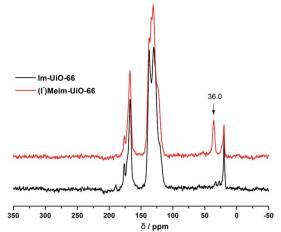
Fig. 2 Solid-state  $^{13}$ C NMR spectra of Im-UiO-66 and (I<sup>-</sup>)Meim-UiO-66
