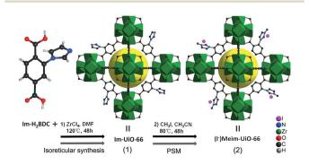
Scheme 1 Syntheses of 1 and 2 via reticular chemistry and by a PSM method, respectively. Green polyhedra: Zr<sub>6</sub> clusters. Yellow ball: micropores. Only part of the linkers are shown for clarity.
