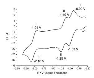
Fig. 3 Cyclic voltammogram for 2 measured as a 1 mM  $CH_2Cl_2$  solution (0.1 M [ $^nBu_4N$ ][BPh $_4$ ] supporting electrolyte, glassy-carbon working electrode, Pt gauze counter electrode and silver wire quasi-reference electrode). Potentials are referenced against the Fc $^+$ /Fc couple measured under identical conditions.
