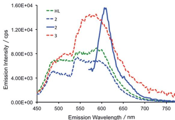
Fig. 6 Emission spectra of HL (green dashed trace), **2** (blue dashed trace) and **3** (red dashed trace) following excitation at 425 nm and the emission spectrum of **2** (full blue line) following 550 nm excitation (298 K, THF). The relative intensities of HL, **2** and **3** are arbitrary with respect to each other.
