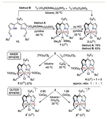
Scheme 1 Synthesis of the uranyl(vı) complexes 1 and 2 and the U(v) complex 3 (isolated yields shown) and reactions between 2 and the inner-sphere reductant,  $[TiCp_2Cl]_2$  and the outer-sphere reductant,  $CoCp_2$ .
