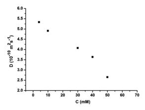
Fig. 3 The concentration dependence of the diffusion coefficient D (400 MHz, CDCl<sub>3</sub>, 298 K) of the mixed solution of 3 and 2 equiv. of 1
