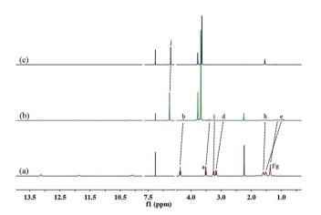
Fig. 1 Partial  $^1$ H NMR spectra (400 MHz, CDCl $_3$ , 298 K) of: (a) 1 (8.00 mM); (b) 1 (8.00 mM) and 2 (12.00 mM); and (c) 2 (12.00 mM).
