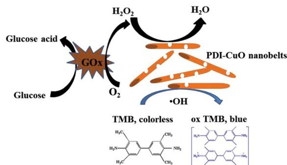
Scheme 1 Schematic illustration of colorimetric sensor for H<sub>2</sub>O<sub>2</sub> and glucose detection using PDI-CuO nanobelts as catalysts.
