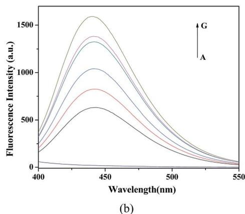
Fig. 8 (a) The reaction of TA with  $\cdot\text{OH}$ . (b) Fluorescent spectra of acetate buffer solution (pH = 4) containing only TA and PDI-CuO (A) or with H<sub>2</sub>O<sub>2</sub> (0.25 M), TA (0.5 mM) and the PDI-CuO nanocomposites with different concentration ((B) 0, (C) 20, (D) 80, (E) 200, (F) 250, (G) 300 μg mL<sup>-1</sup>) were incubated at 55 °C for 30 min. The FL excitation wavelength was fixed at 315 nm.
