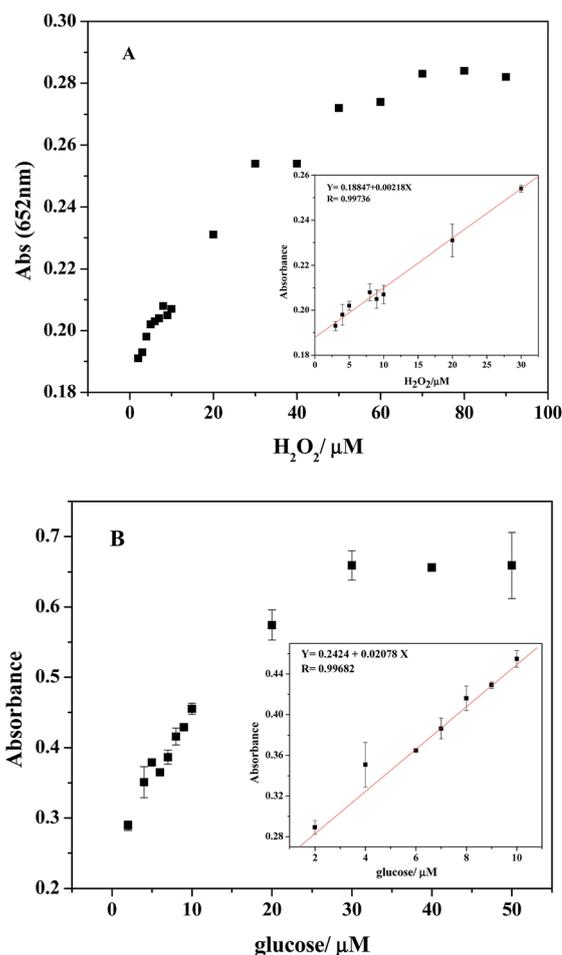
Fig. 9 (A) A dose-response curve for H<sub>2</sub>O<sub>2</sub> detection using PDI-CuO under the optimum conditions. Inset: the linear calibration plot for H<sub>2</sub>O<sub>2</sub> detection (B) A dose-response curve for glucose detection using PDI-CuO as catalysts. Inset shows the linear response of the detection system to glucose. Error bars stand for the standard deviations based on three repeated measurements.
